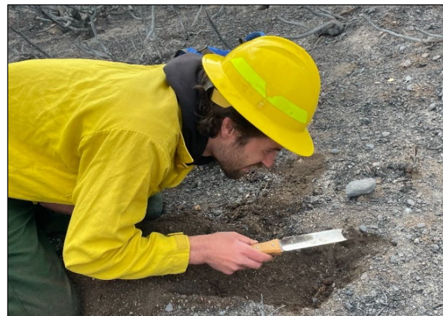
Nathan Clark, soil scientist on the Davis Fire BAER Team, dug a small pit to look at the soil burn severity by studying the surface soil structure, root conditions, and water repellency.
